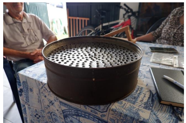
Fig. 15. The grater used to calibrate the couscous grains (Photography: Author 1).
